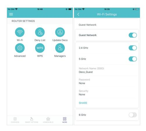
Manage guest network (e.g. change the Wi-Fi name and password, hide the network from Wi-Fi list, set channel width for 5GHz Wi-Fi. etc.).
